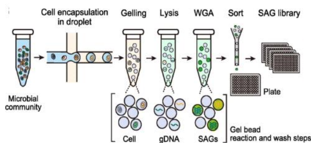
Fig 1. Workflow for SAG-gel-based single-cell genome sequencing. 1)
